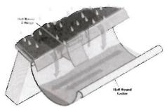
4900 Half Round T-Wedge supports 6 inch half round gutters in any slanted or sloped application including crown molding, 1×2 trim board, etc. Uniquely designed for simple installation and is totally adjustable.
